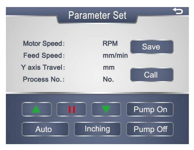
Press the **Parameter** key to enter the parameter setting interface. This menu controls all operating values that determine cutting speed, travel distance, and motion behavior. Accurate parameter entry is essential for achieving consistent and repeatable results.
