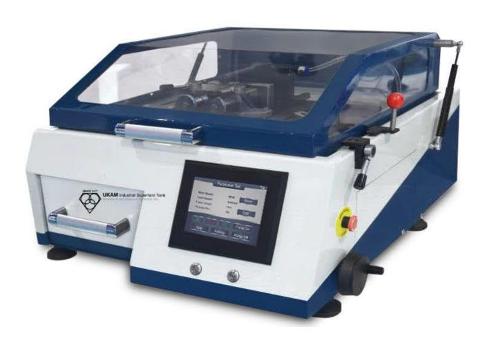
**SMART CUT® 6018** is a precision benchtop sectioning saw designed for accurate and repeatable cutting of many laboratory and production materials. The machine uses a **speed regulation motor** that drives the belt to control the cut off wheel. This provides **stable and efficient spindle speed** for both hard and delicate samples. The system is operated through a **touch screen interface** with a clear display and organized control layout.
