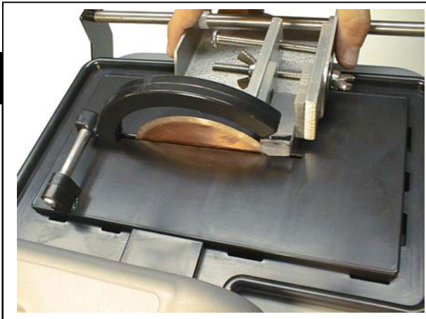
Operator can change blade speed (RPM's) during operation.
