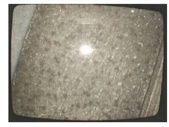
Diamonds are placed inside bond with no control over diamond distribution or orientation. 100 concentration is used to make sure the blade will cut hard materials.
